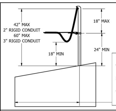
18 INCH MINIMUM CLEARANCE ABOVE ROOF INCLUDING SERVICE WIRES AND DRIP LOOP
